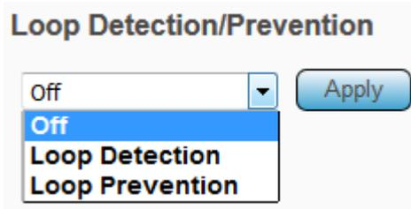
Loop Detection: the LINK/ACT LED will blink in a regular time (about 1s).
