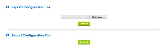
Here, the AP's current settings can backed up and exported to a file or restore previous settings by importing from a previously backed up configuration file. If importing, the device will restart and apply the new settings.
