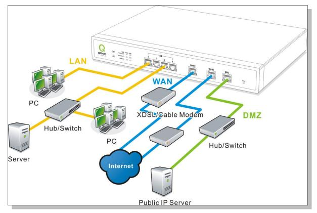
**WAN connection** : A WAN port can be connected with xDSL Modem, Fiber Modem, Switching Hub, or the Internet through an external router.
