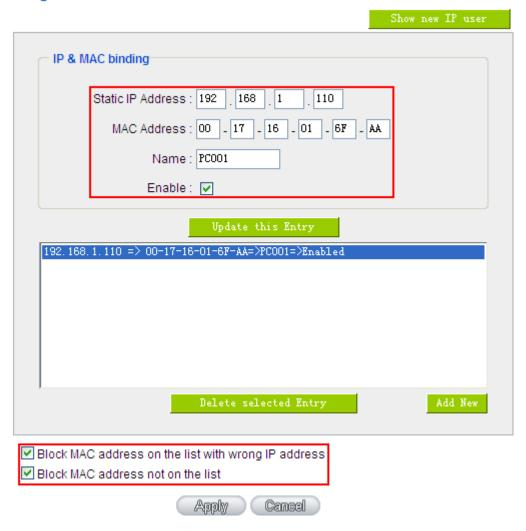
After an item is added to the list, the corresponding message will be displayed in the white block on the bottom. However, such method is not recommended because the inquiry of IP/MAC addresses of all hosts creates heavy workload. Another method to bind IP and MAC is more recommended because of easy operation, reducing workload and time efficiency. It is described in the following.
